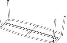
Turn the frame with the legs upside down. Fasten the suction cups onto the frame as shown in the picture below. The frame has holes in wich you can fasten the threaded suction cup.
