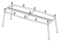
Put the table frame upside down onto the table top. The table top is marked where the suction cups should be positioned.
