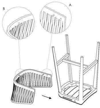
Attach the Back part to the seat part using 1 x washer, 1 x nut and an adjustable spanner.
