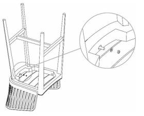
3 Use 2 x screw, 2 x washer and an Allen key to connect the Back part to the Seat part on the front side of the chair.
